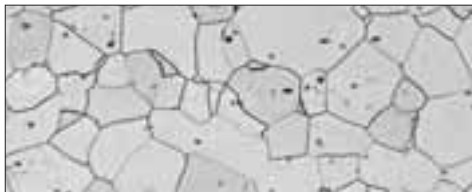
Figure 1.2. The microstructure of a ferritic stainless steel
