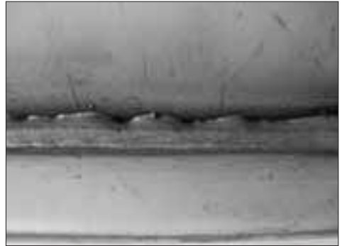
Figure 5.1. Lack of fusion – MIG
