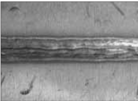
Figure 4.6. Stringer beads in PC position
