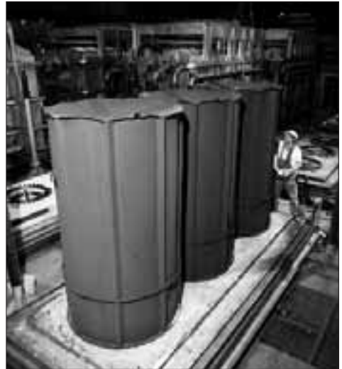
Figure 6.4. Bell furnaces for heat treatment in 253 MA
