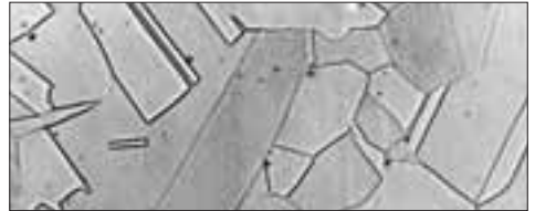
Figure 1.6. The microstructure of an austenitic stainless steel
