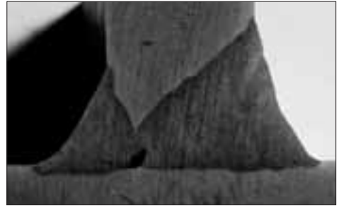
Figure 5.6. Slag inclusion in a 2205 FCA weld
