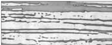
Figure 1.10. The microstructure of a duplex stainless steel
