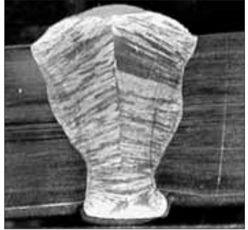
Figure 5.12. Excessive weld metal – MIG 316L-Si
