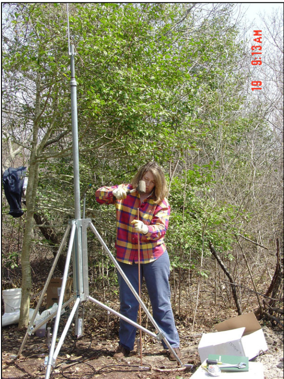
Left: Carolyn Bishop (INEEL) installs the Site D hydrology station with three tensiometers, a thermocouple and a reflectometer. A solar panel will provide recharge capability for the data logger (April 2004).
