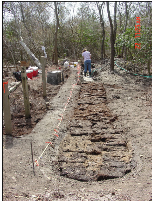
Left: Carolyn Bishop (INEEL) installs the Site D hydrology station with three tensiometers, a thermocouple and a reflectometer. A solar panel will provide recharge capability for the data logger (April 2004).
