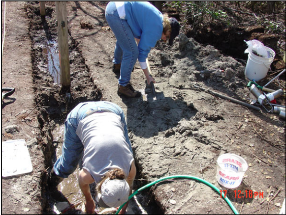
Above Left: In the trench, Kay Adler Flitton (INEEL) and to the right of the trench, Kathy Marshall (SRTC), work on removing overburden, pumping groundwater, and sampling soil and ground water during coupon recovery (April 2004).
