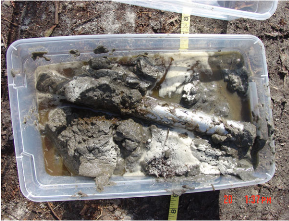
Above Left: 409 stainless steel pipe sample upon recovery (April 2004).
