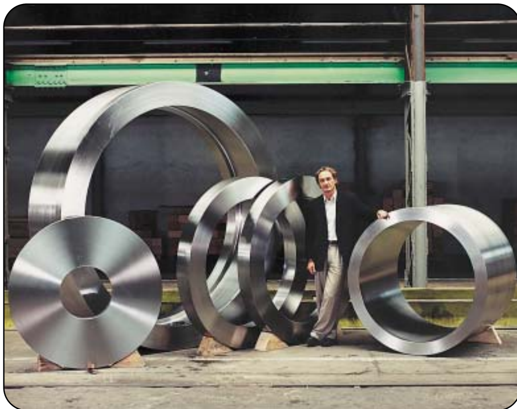
Rings and discs made of duplex and super duplex grades for offshore application
