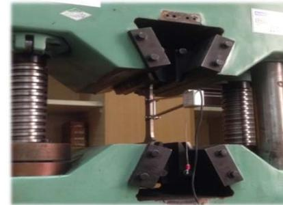
b. Test configuration of tensile test
