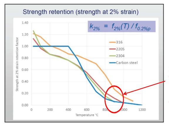
Zone of interest for the products presented as designs ensure that none are load-bearing during a fire
