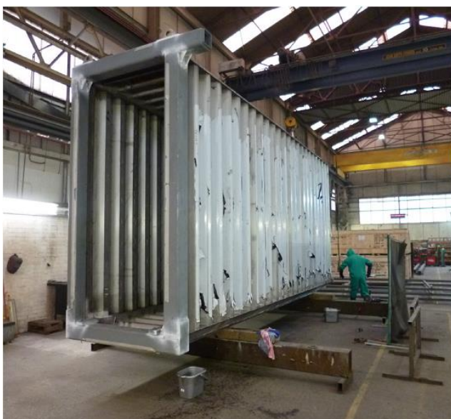
Fig. 33 A section of a stainless steel escape tunnel carcass in construction in UK with a carbon steel support ring frame attached by welding and fire protected with intumescent PFP at site.
