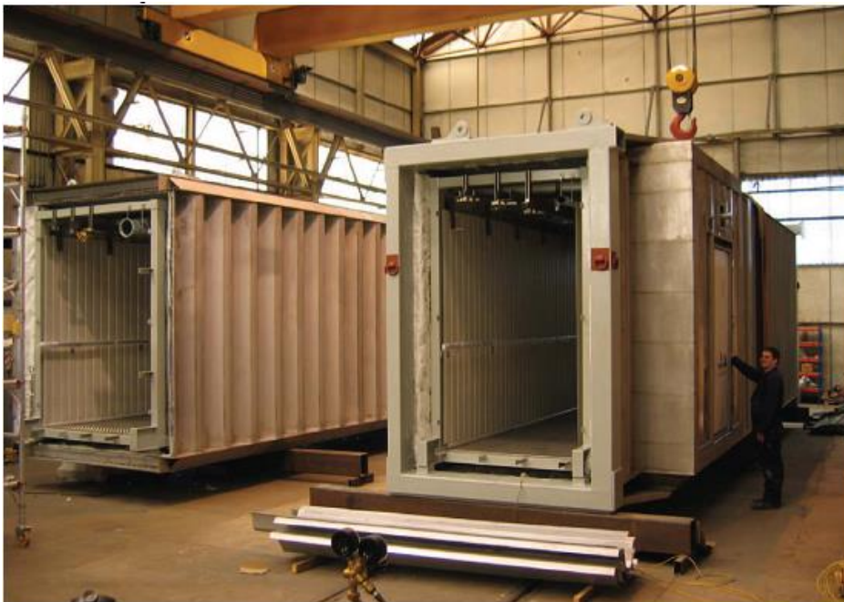
Fig. 34 Section of a type 2 FPSO escape tunnel, note door to the side. This communicates with a stainless blast resistant airlock room sited on the deck of the FPSO.
