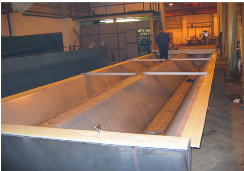
Fig. 11 Prefabricated Duplex stainless steel prefabricated panel ready for shipment to Australia part of a 13 m high blastwall).
