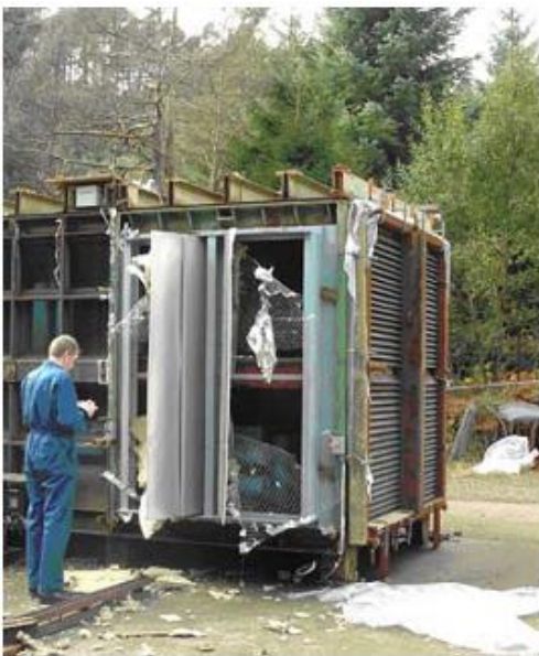
Fig. 28 Explosion Relief panel after explosion test to 0.5bar.
