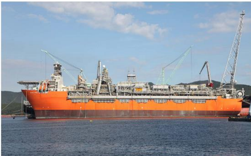
Fig. 31 An FPSO (Floating Production, Storage & Offloading platform) for Norwegian N Sea Note Stainless Steel Fire and blast resistant escape tunnel all along the side.
