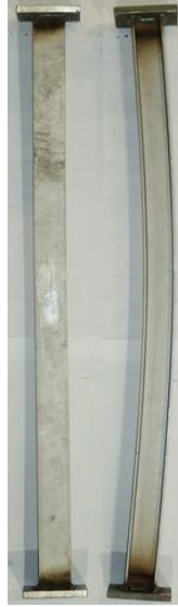
Fig. 10 Typical failure mode for beam-column under combined axial compression and bending about the major axis (50Maj5)
