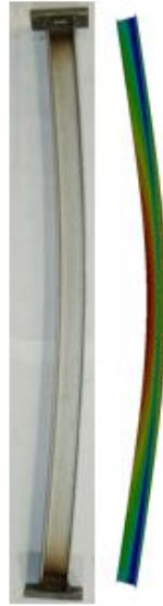
Fig. 12 Experimental and numerical failure modes for beam-column specimen 50Maj5 under compression and bending about the major axis
