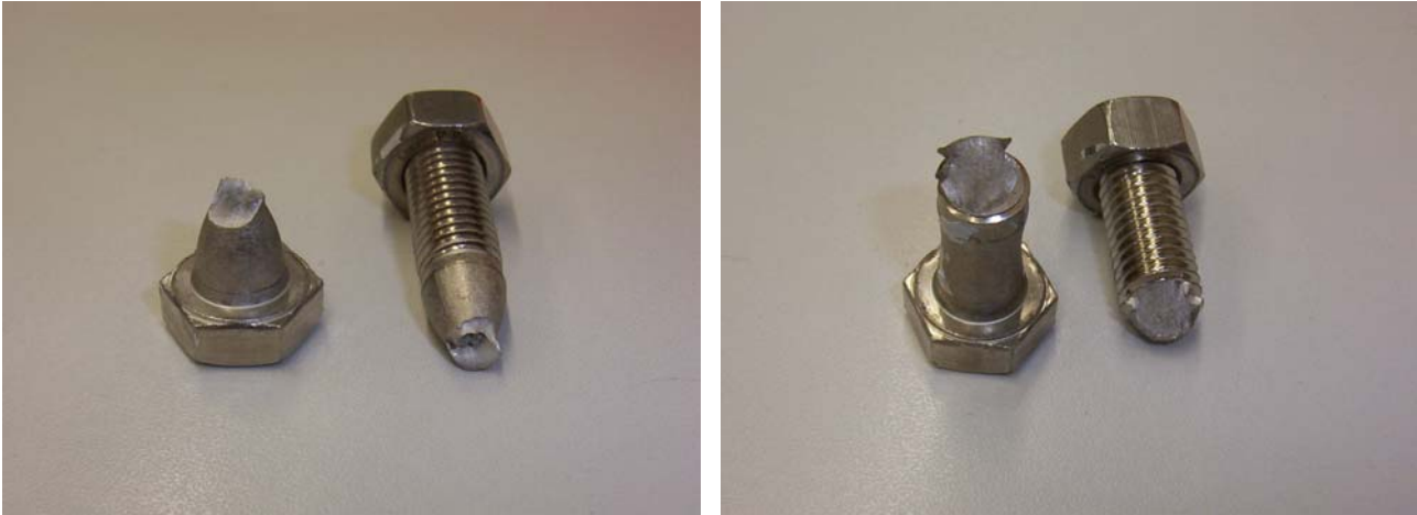
Figure 4 – A4 80 bolts different failure modes at T = 300 °C.
