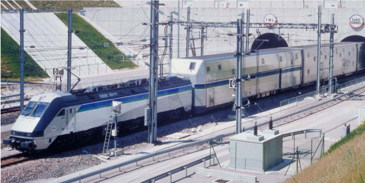
Fig. 3. Eurotunnel shuttle cars. Locomotive is of standard size. (Courtesy of Nickel Institute)
