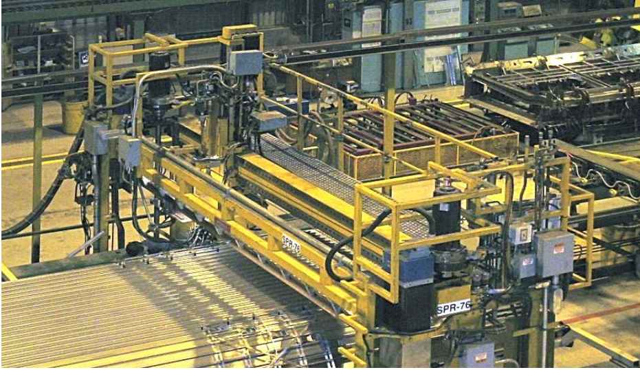
Fig. 8 Station for welding large sides and roof panels (Bombardier)
