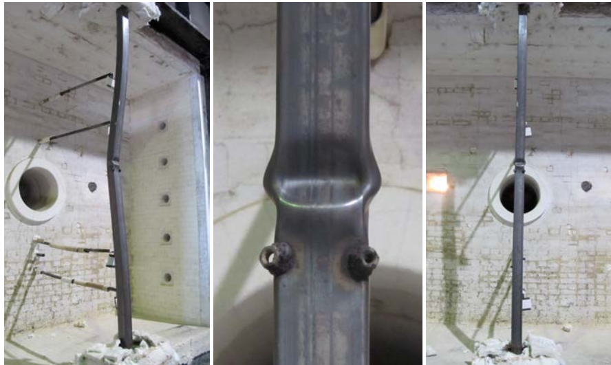
Figure 5. Failure mode for the specimen # 1 (3m long).
