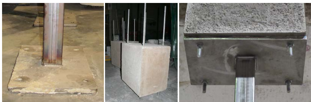
Figure 4. Left to right – bottom end plate with holes for bolts, supporting concrete block with waiting steel bars, column top end with plate mounted on concrete block.
