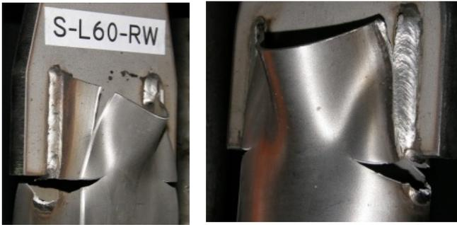
**Fig. 6. Typical deformed shape for short and medium weld length connections**
