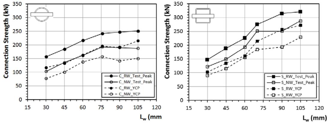
**Fig. 11** Variation of connection yield capacity point,  $Q_y$  and test peak strengths,  $N_{test}$  with weld length,  $L_w$
