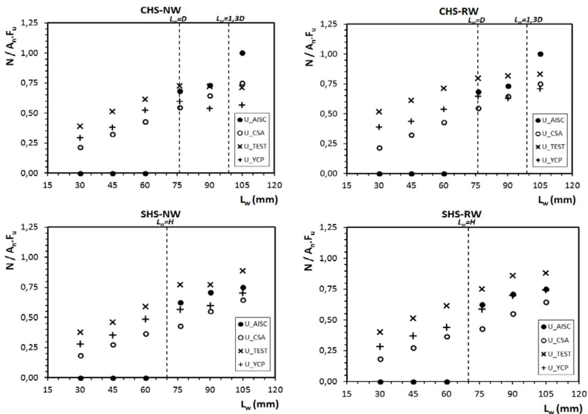
**Fig. 12 Comparison between the test and code predicted efficiency factors for all the test specimens**
