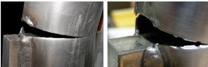
**Fig. 7 Failure types for return weld (RW) and no-return weld (NW) cases**
