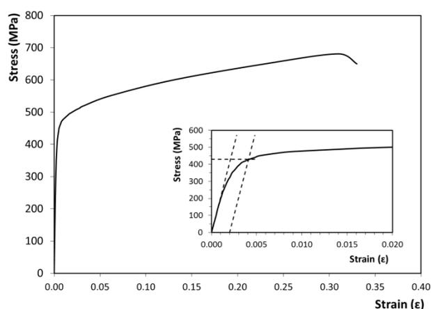
**Fig. 4. Typical stress–strain curve from tensile coupon tests**
