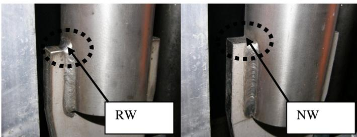
**Fig. 3. View of the slot end conditions with / without a return weld**
