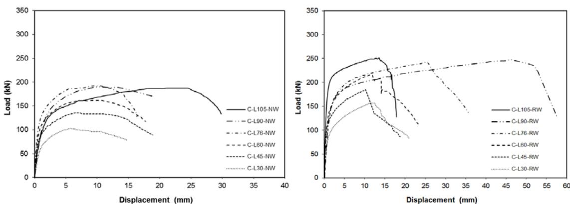
**Fig. 8 Load-displacement curves for the ‘With return weld (RW) and No Return weld (NW)’ specimens for Circular Hollow Sections**
