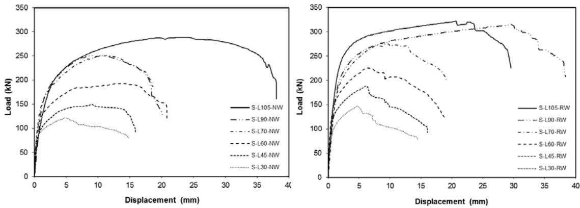
**Fig. 9** Load-displacement curves for the ‘With return weld (RW) and No Return weld (NW)’ specimens for Square Hollow Sections
