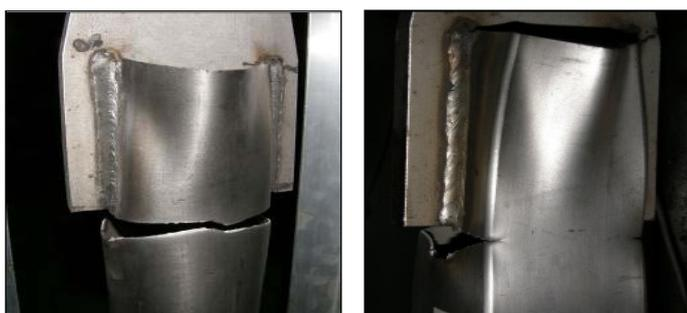
**Fig. 5. Typical deformed shapes observed for CHS and SHS members with long weld lengths**
