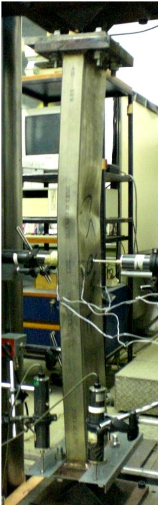
Fig. 3. Interaction of local and flexural buckling in test and FEA of specimen C6L900
