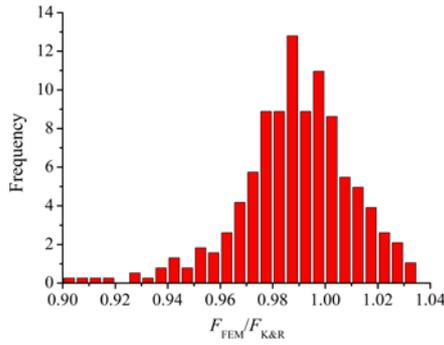
**Fig. 6 Comparisons of the strength predicted using Method proposed by Rasmussen and finite elements results**
