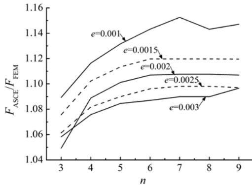
**Fig. 5 Comparisons of the strength predicted using American specification and finite elements results**
