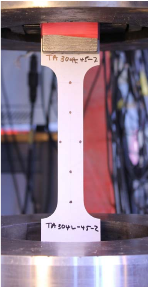
Figure 10 Typical tensile coupon (TA-45-2)
