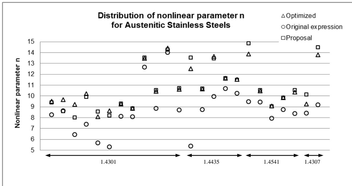
**Figure 4** Experimental and analytical nonlinear parameter n values for austenitic stainless steels
