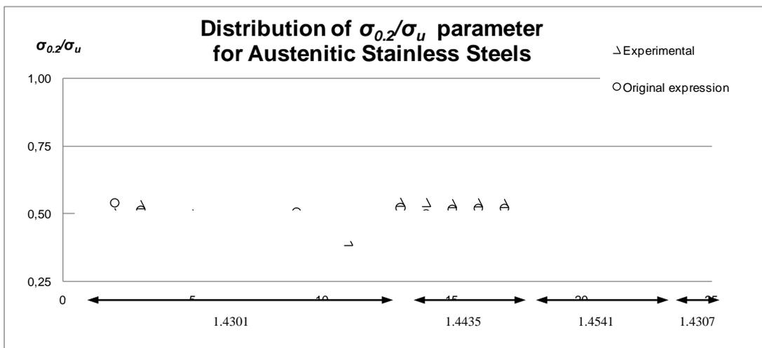
Figure 6 Experimental and analytical  $\sigma_{0.2}/\sigma_u$  values for austenitic stainless steels.
