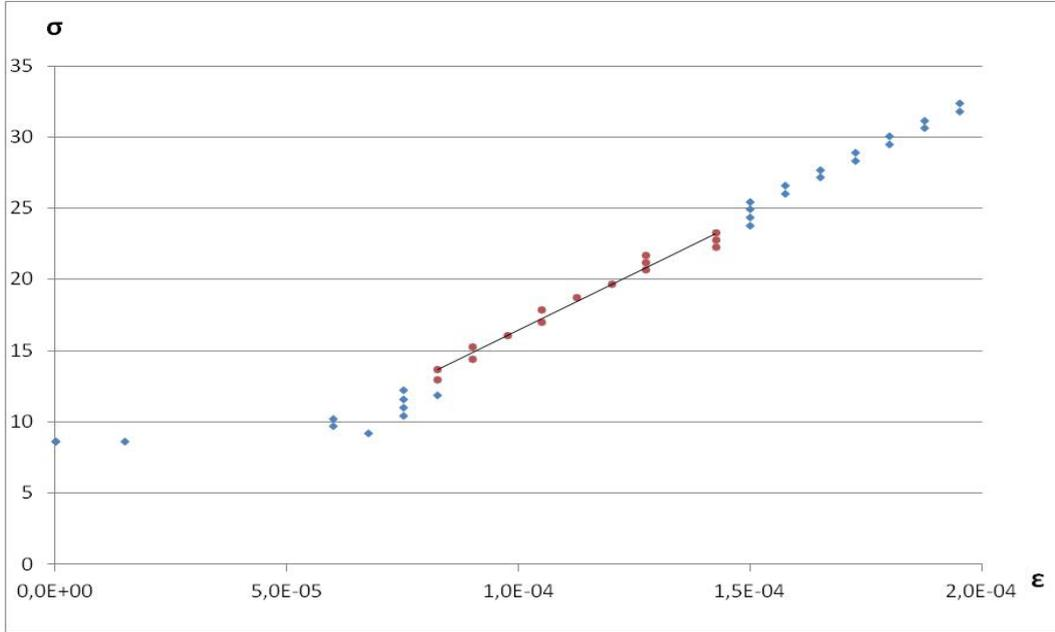
**Figure 1 First point selection for the initial modulus determination**
