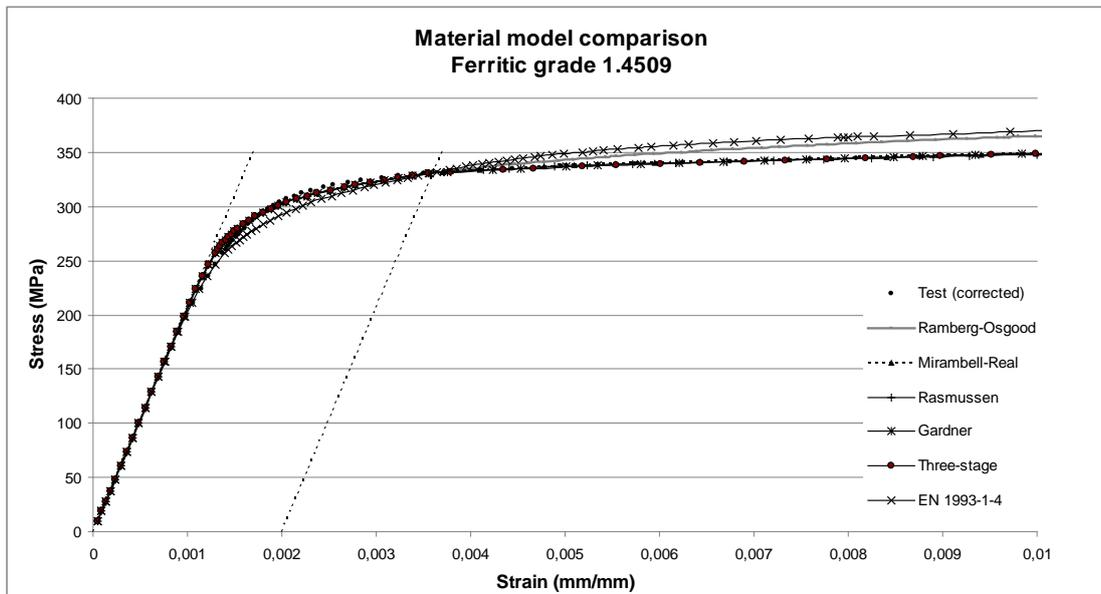
**Figure 3** Experimental and optimized stress-strain curves for a ferritic grade 1.4509 coupon test.
