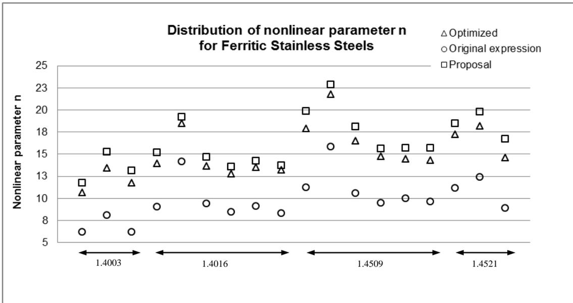
Figure 5 Experimental and analytical nonlinear parameter  $n$  values for ferritic stainless steels.
