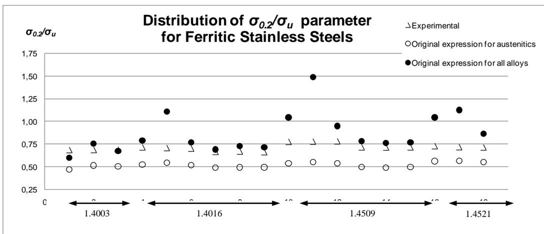
Figure 7 Experimental and analytical  $\sigma_{0.2}/\sigma_u$  values for ferritic stainless steels.
