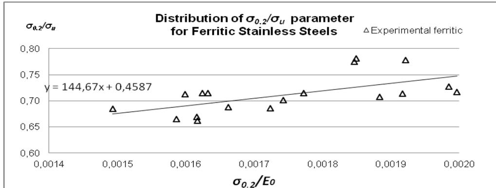
**Figure 8** Linear approximation for  $\sigma_{0.2}/\sigma_u$  values for ferritic stainless steels.
