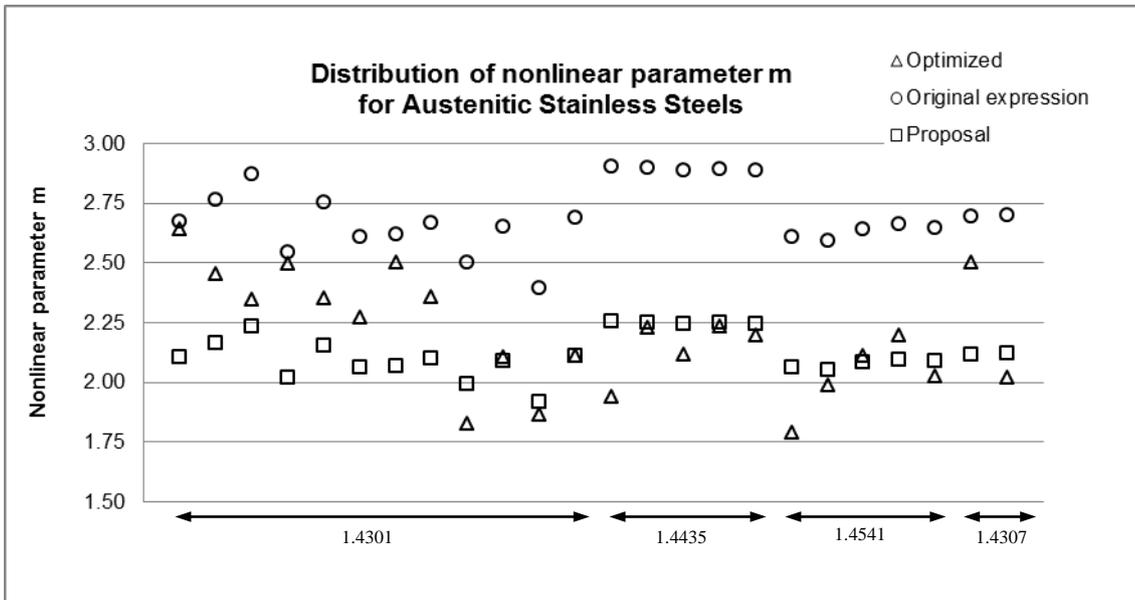
**Figure 9** Second nonlinear parameter  $m$  experimental and analytical (original expression and new proposal) values for austenitic stainless steels.
