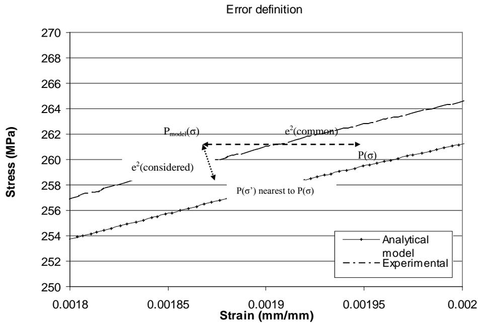
**Figure 2. Error considered in the nonlinear parameter optimization.**
