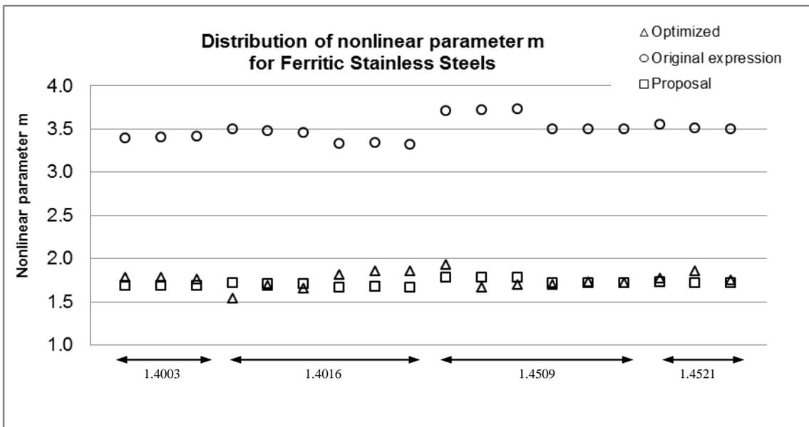
**Figure 10** Second nonlinear parameter  $m$  experimental and analytical (original expression and new proposal) values for ferritic stainless steels.
