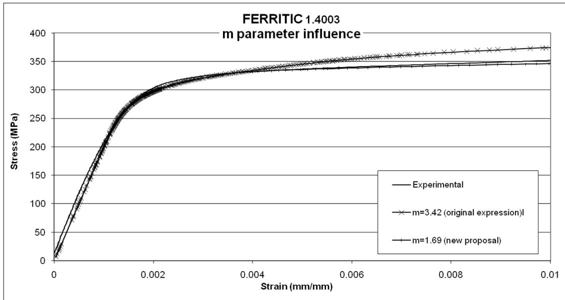
**Figure 11** Stress-strain curves for the original and proposed  $m$  expression for ferritic grade 1.4003.
